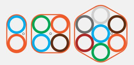
Höhle microducts are designed for long term protection of fiber optical cables. Direct Bury (DB) type of microducts are thick wall products that attain their mechanical robustness and functional performance through their intrinsic thick walls and need no further protection at underground installations.
